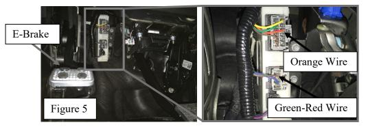
Attached 6" wire between Orange wire(Pin 3 on C2498C Connector) and Green-Red wire (On F150) or Red wire (on Super Duty) (Pin 1 on C2498A Connector) using Scotchloks (For F150 supplied Scotchloks can be used, Super Duty are not supplied, recommend using 3M 902). This will activate a continuous +12V to the +12V power pin on the 7pin trailer connector. Refer to Figure 6
