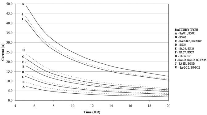
\* Above values are to 90% SOC (State of Charge) based on C100 Ah capacity
