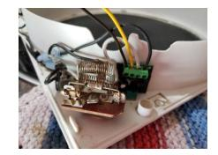
6. Back to wiring... I made two pigtails one Yellow and one Black with appropriate Male and Female spade connectors on each so they could plug into the FWC power wires I previously added connectors to and determined polarity. The opposite end of each pigtail was stripped ¼ " to be inserted into the PWM. The Black is inserted into the POWER negative (-) and the Yellow into the POWER positive (+)
