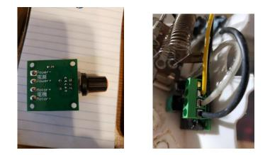
7. There are two wires connected to the REVERSE switch one is Black negative (-) and the other White positive (+). Those wires come from the 3-speed controller switch. I once more cut the wires and added blade connectors so polarity can not be mixed. I made two more pigtails one white and one black. Crimped on appropriate blade end male and female then stripped the opposite ends ¼ ". These ends are inserted into the PWM on the MOTOR connection BLACK to negative (-) and White to positive (+)
